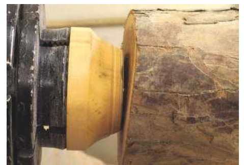
▲ Pic.2 Cut the wood off at 60mm and drill a 3mm hole in the end; when you screw the wood onto the chuck make sure it's right up against the face of the chuck or risk breaking the screw
